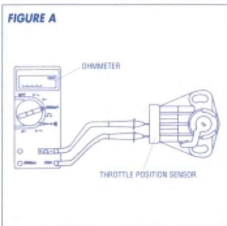
Next, connect the ohmmeter between the center terminal and the other outer terminal. Repeat the same test. The ohmmeter reading should again rise or decrease smoothly as you exercise the sensor.
