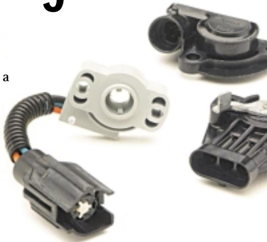
One of these is the Throttle Position Sensor (TPS), which tracks the opening and closing of the engine's throttle.
