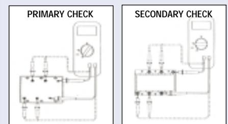
In most cases, you'll find a coil where the secondary resistance is reading too high. Some coils may also test okay when cold, but be out of specifications when the coil heats up.
