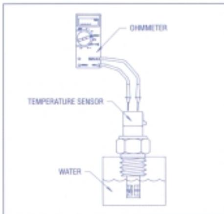
To test the sensor, remove it from the manifold and connect an ohmmeter across the terminals. Alter the sensor's temperature by immersing the tip of the sensor in either warm or cold water.
