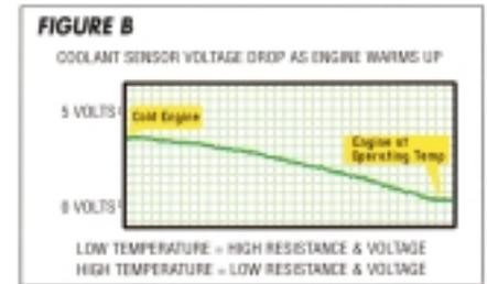
If a vehicle provides live sensor data through its diagnostic connector, you can also read the coolant sensor's output directly with a scan tool (usually in degrees Centigrade or Fahrenheit).
