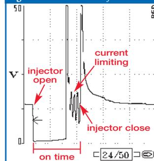
The fuel injector driver opens the fuel injector by holding the circuit to ground until the injector has 3.5-4.0 amps flowing through it.
