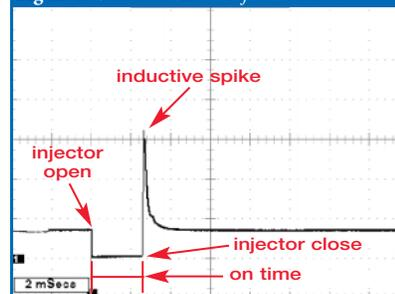
When the fuel injector driver turns the circuit OFF by removing the ground, an inductive spike is produced as the magnetic field surrounding the fuel injector windings collapses. This spike is captured by the oscilloscope as a vertical line. A fuel injector with shorted windings will shorten the spike (reduced amplitude). Injector pulse width, or ON time, can be determined by measuring the time the oscilloscope trace remains at 0 volts.
